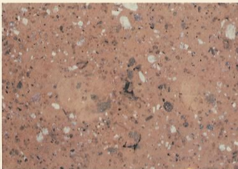
Figure 24. Micrograph ( \times 3 ) of Nagasaki Ieno-cho brick sample NA1E08.
