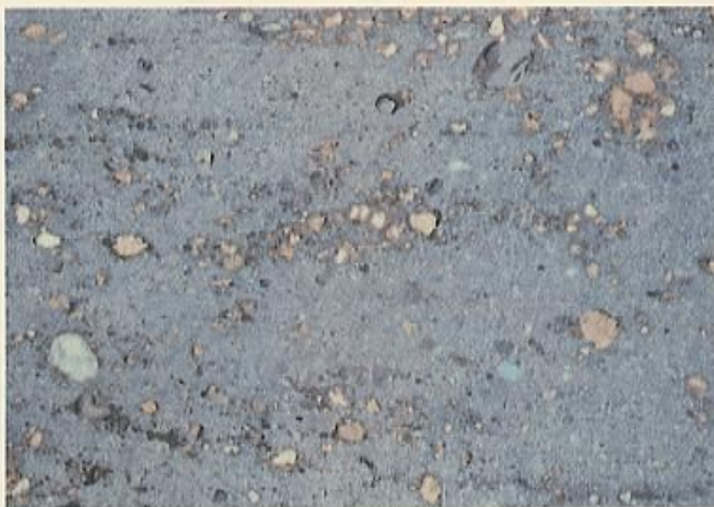
Figure 25. Micrograph ( \times 3 ) of Hiroshima University tile sample UHFS03.
