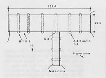
Figure 1. Plan for the Aioi Bridge. Lengths are shown in meters. A-1 to A-3 and B-1 to B-3 show the places where the materials were collected. 5,6
