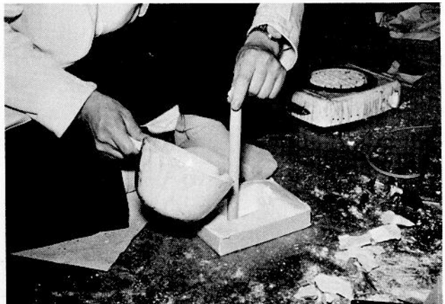
Figure 3 Filling mold with Mix-D material, reserving a place for ionization chamber in the bone.
