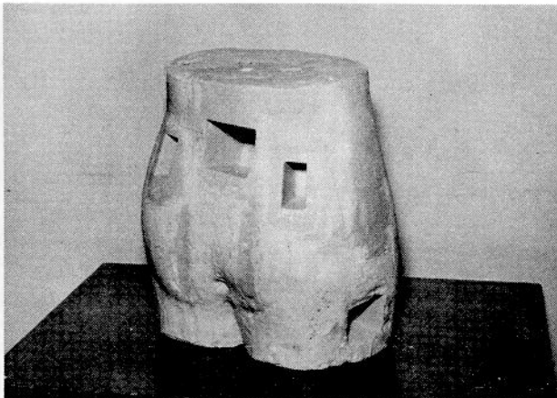
Figure 6 Abdomen and pelvis section of phantom with receptacles for drawers accommodating ionization chambers.
