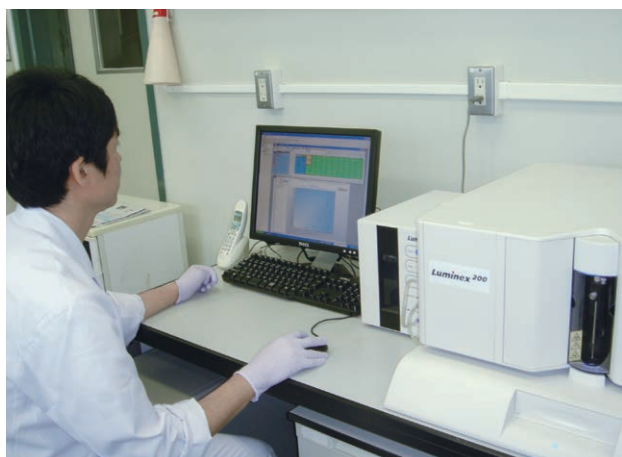
Luminex Complete System 200 (fluorescent microbead array system). This system made it possible to measure multiple cytokines simultaneously using limited sample volume (serum, plasma, etc.) by the multiplex bead array assay.
