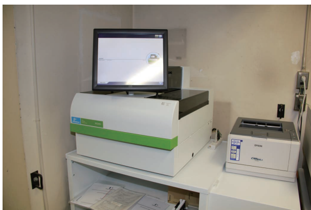
2470 Wizard 2 Gamma Counter 3.0 inch well-type NaI(Tl) gamma counter. This device provides improved counting efficiency, extended energy range, and better energy resolutions for gamma emitting radionuclides such as ^{125}\text{I} and ^{51}\text{Cr} . It is used for protein labelling in biomedical research and also for monitoring of environmental contamination.
